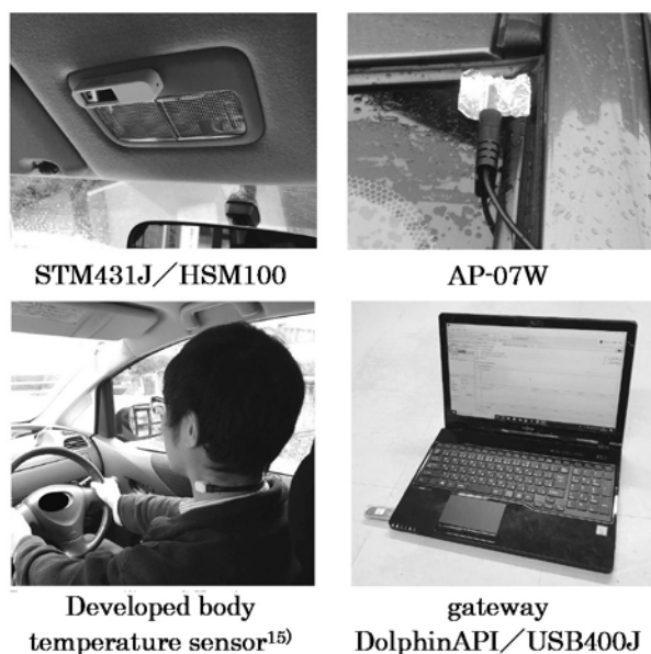
Fig. 2 Pictures of installed sensors
